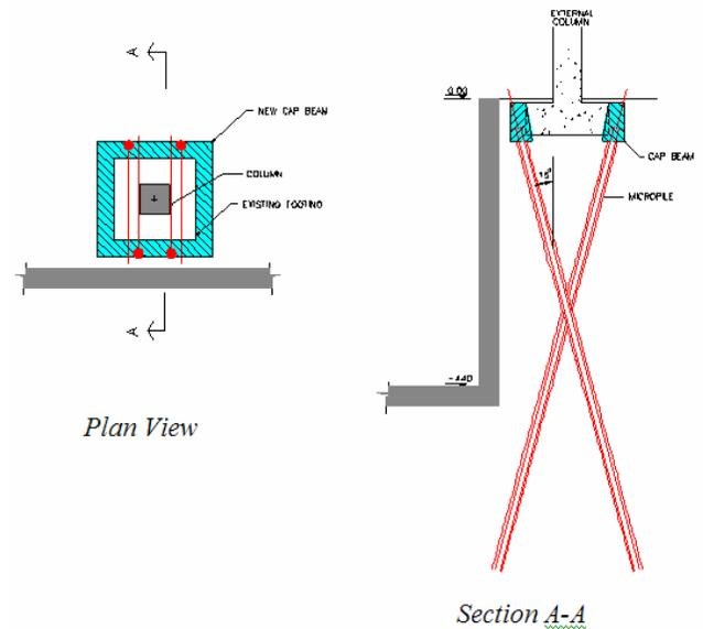
Fig. 4. Detail of micro-piles used for underpinning
